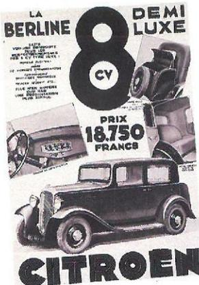
lie. "Floating power" engine of 1,452 cc, 32 bhp at 3,200 rpm, 8 CV. Three-speed gearbox with synchromesh on second and third, 90 km/hour (56 mph), 9.0 litres/100 km (31 mpg). Built as Torpedo, saloon, and 2 or 4-seat convertible, with 38,835 produced between October 1932 and January 1935.
