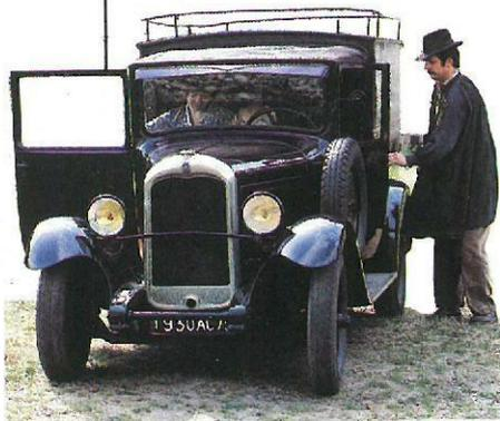
Maximum speed 90 km/hour (56 mph), 8.8 litres/100 km (33 mpg). Developed from the C4 Familiale, this model is equipped with folding back seats and a two-section rear door.
