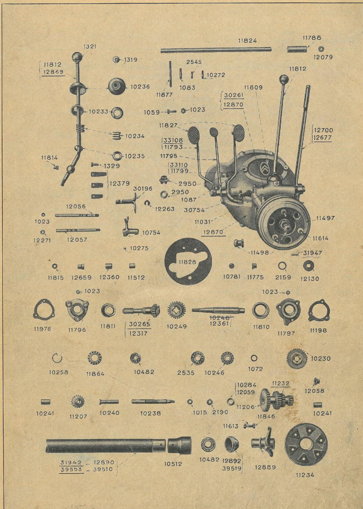
BOITE DE VITESSES (DIRECTION A GAUCHE), TUBE DE REACTION
