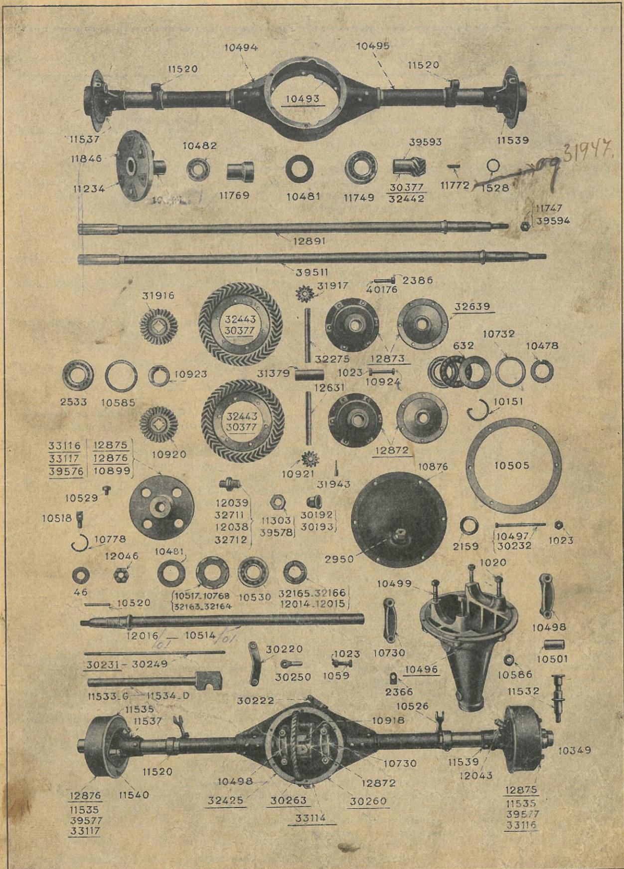
PONT ARRIERE, ARBRE DE TRANSMISSION (POUR TUBE DE REACTION, VOIR PLANCHE 5)
