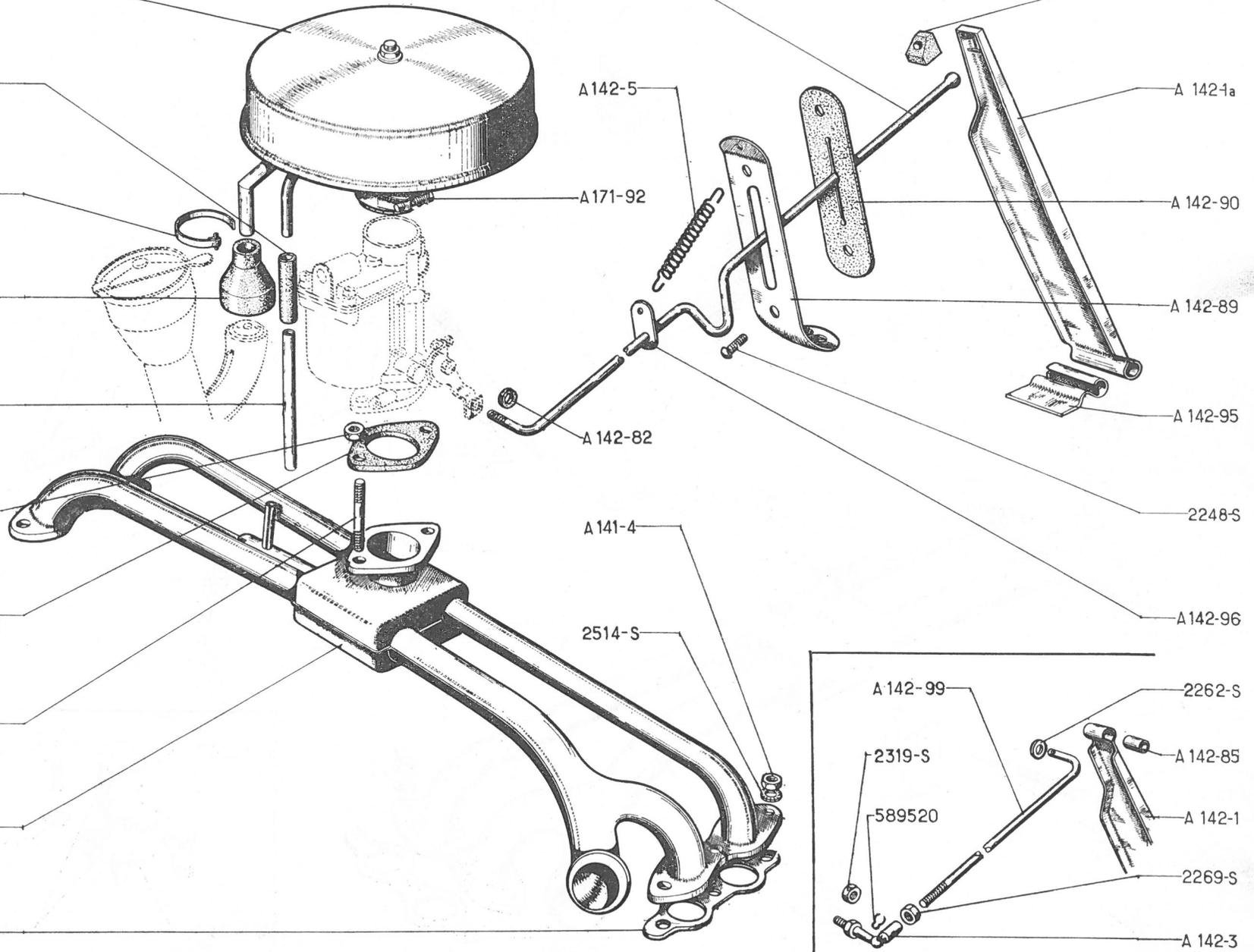
20 — TUBULURE - COMMANDE D'ACCÉLÉRATEUR - FILTRE A AIR AZ-AZU
