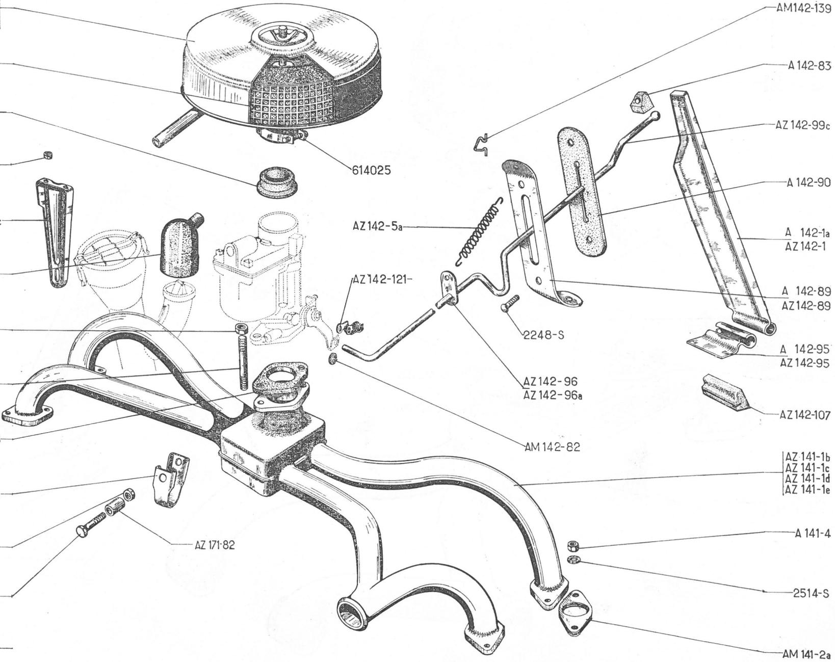
24 — TUBULURE - COMMANDE D'ACCÉLÉRATEUR - FILTRE A AIR AZU
