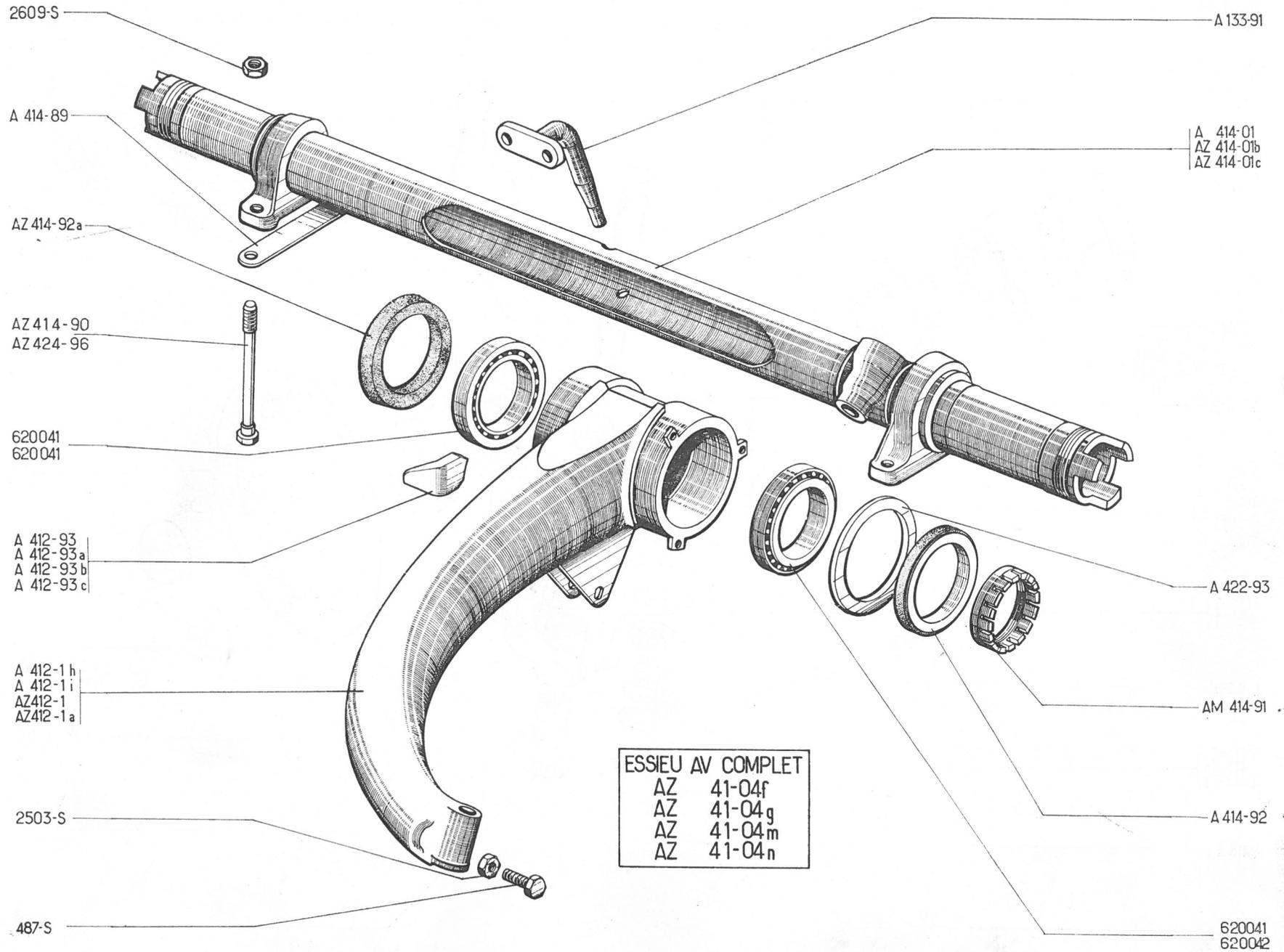
64 — ESSIEU AV - PIVOTS - MOYEURS - LEVIERS D'ACCOUPEMENT
