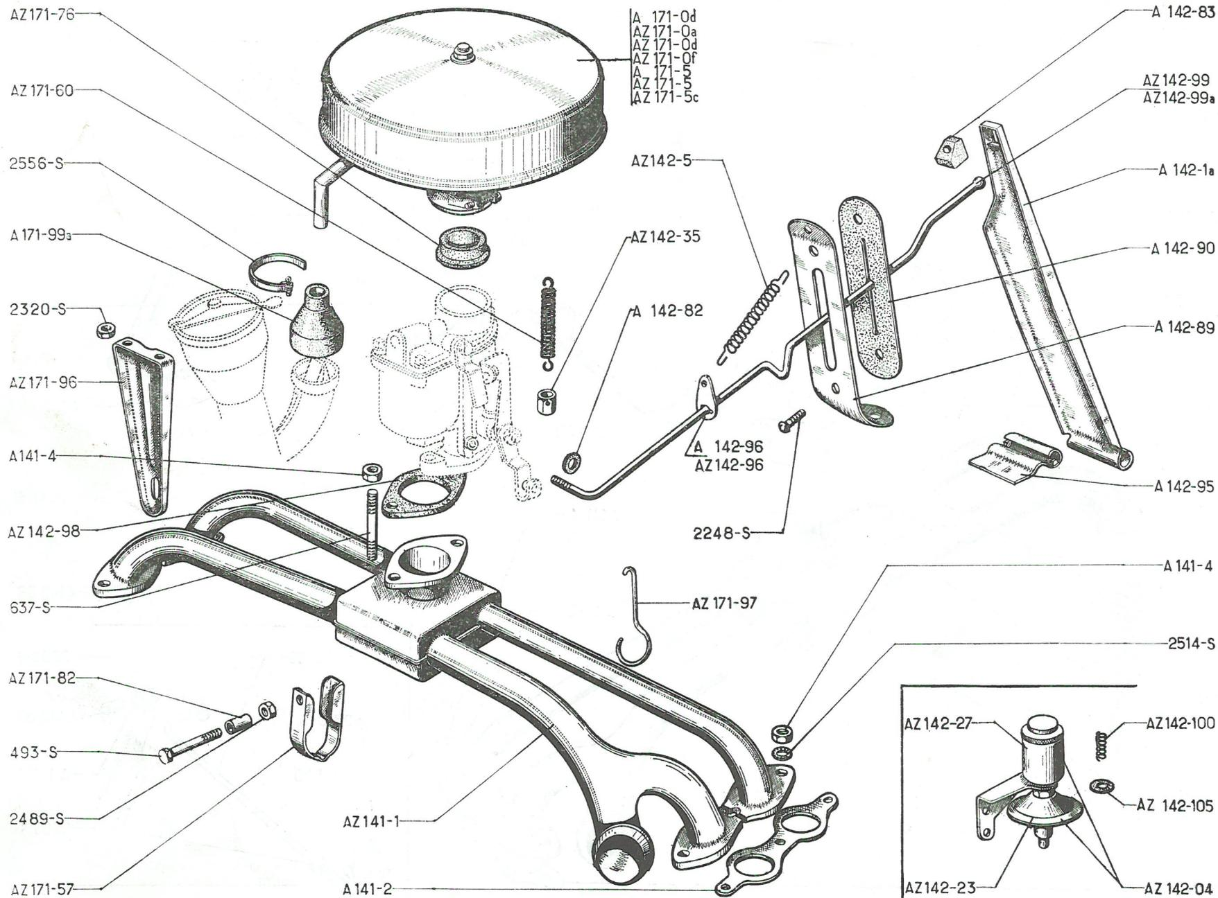
TUBULURE - COMMANDE D'ACCÉLÉRATEUR - FILTRE A AIR AZ-AZU — 21
