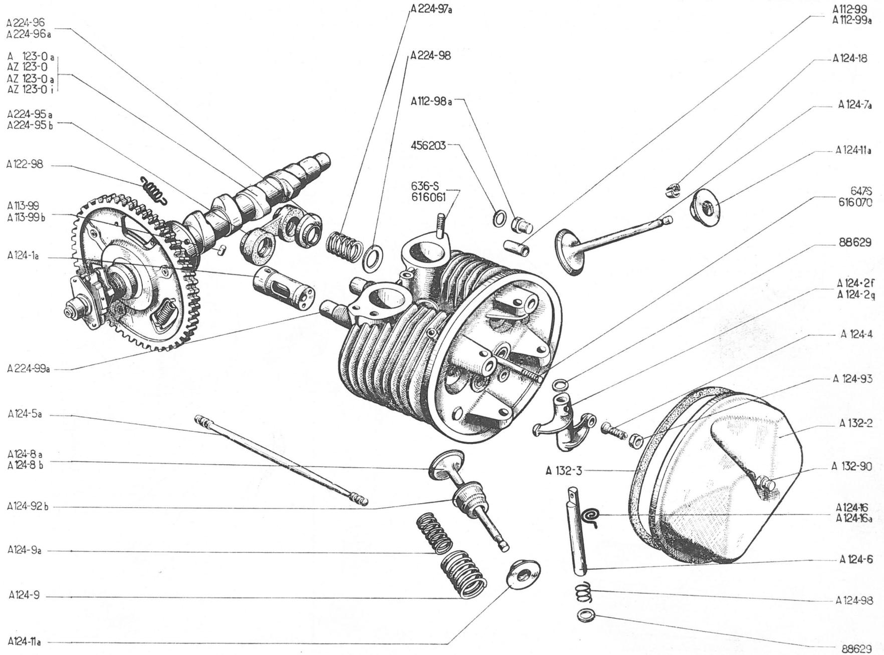
16 — ARBRE A CAMES - CULASSES - SOUPAPES - CULBUTEURS - COUVRE-CULASSES
