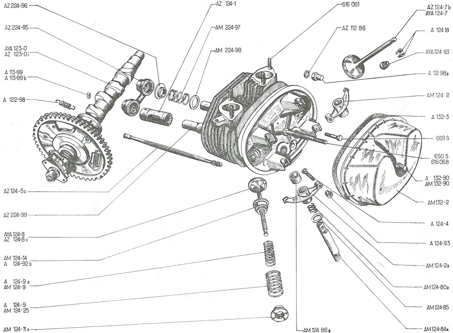
**ARBRE A CAMES - CULASSES - SOUPAPES - CULBUTEURS - COUVRE-CULASSES — 17**
