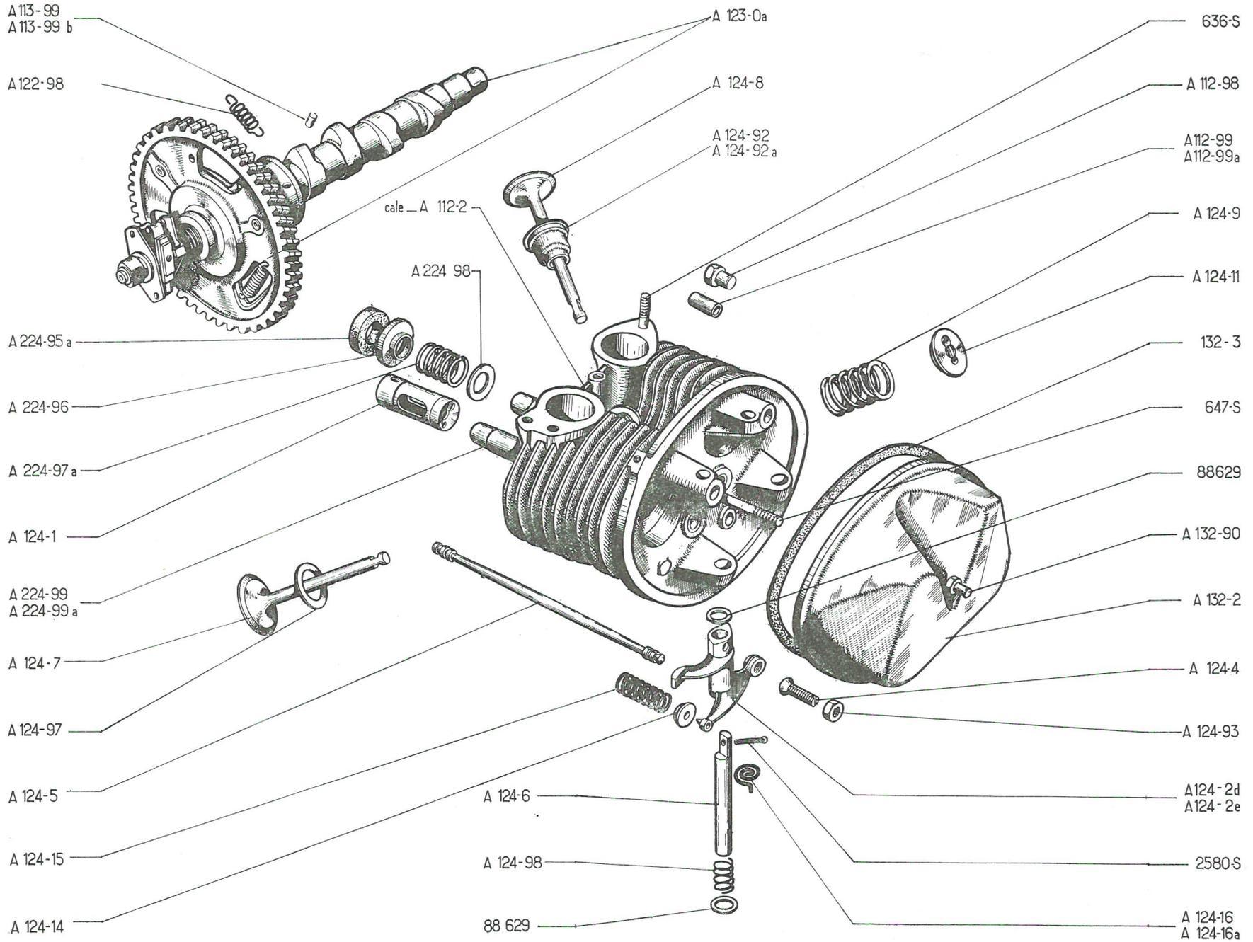
**ARBRE A CAMES - CULASSES - SOUPAPES - CULBUTEURS - COUVRE-CULASSES — 13**
