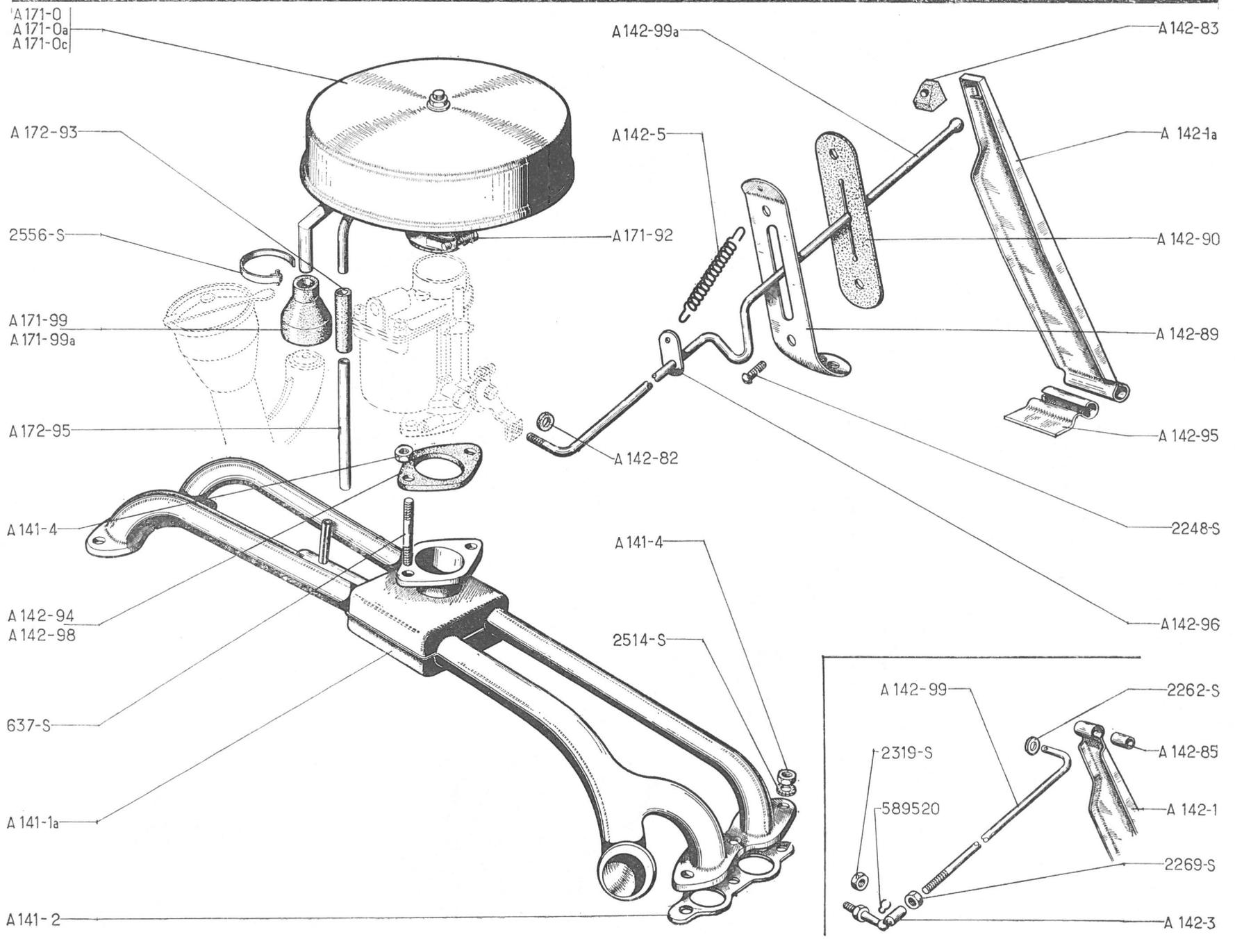
20 — TUBULURE - COMMANDE D'ACCÉLÉRATEUR - FILTRE A AIR AZ-AZU
