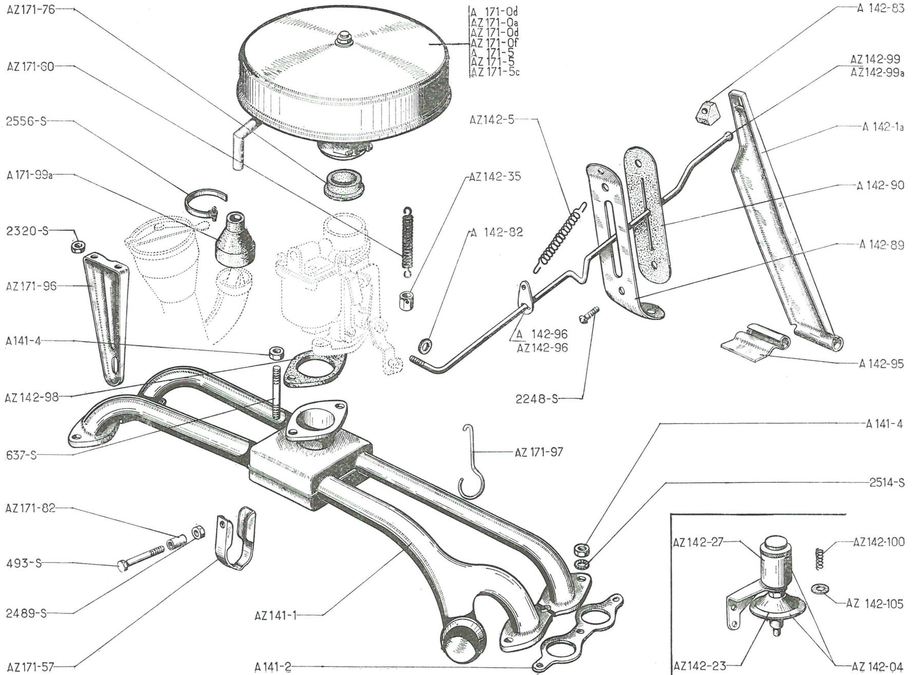
**TUBULURE - COMMANDE D'ACCÉLÉRATEUR - FILTRE A AIR AZ-AZÜ — 21**
