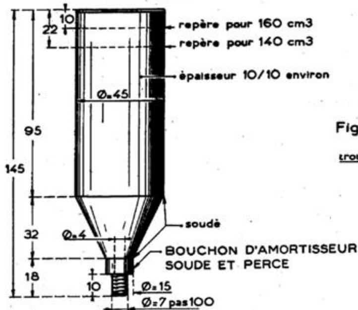
Fig 3 - GUIDE DU CLAPET
