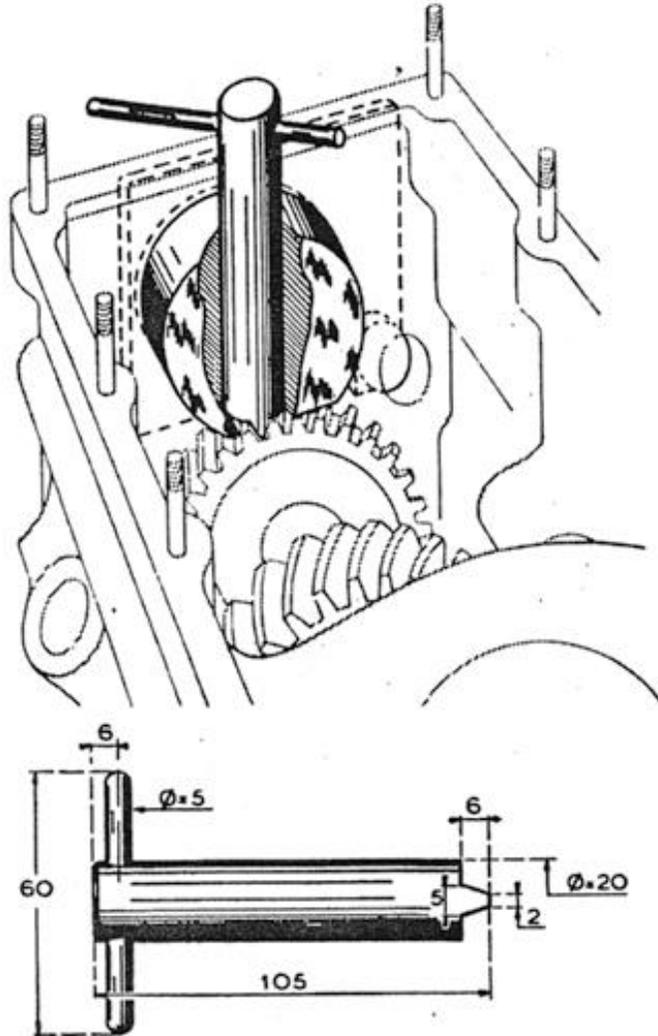
Fig.2 - APPAREIL DE MAINTIEN MR-3139
