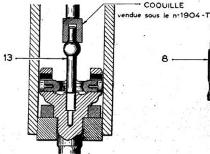
Fig.15\_MISE EN PLACE DE LA MACHOIRE DOUBLE SUR LA FUSEE
