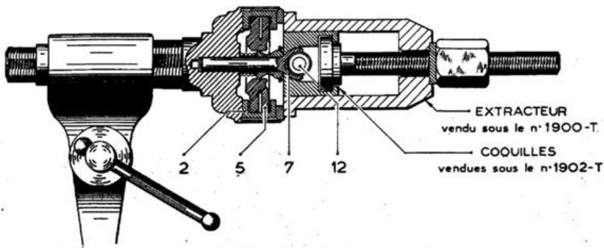
Fig. 7 \_ EXTRACTION DE LA ROTULE D'ARBRE DE TRANSMISSION
