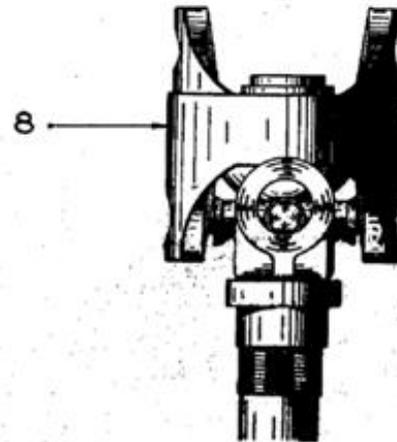
Fig.16\_MISE EN PLACE DE L'ARBRE DE COMMANDE SUR LA MACHOIRE
