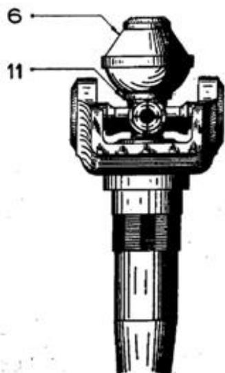
Fig. 6 \_ EXTRACTION DE LA ROTULE DE FUSEE
