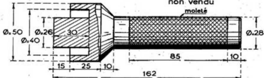
Fig 5 - CLES POUR VIS DE FIXATION
