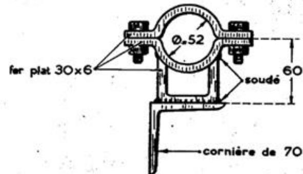
Fig. 1 - CLES POUR TUBE DE MAINTIEN DES NOIX
