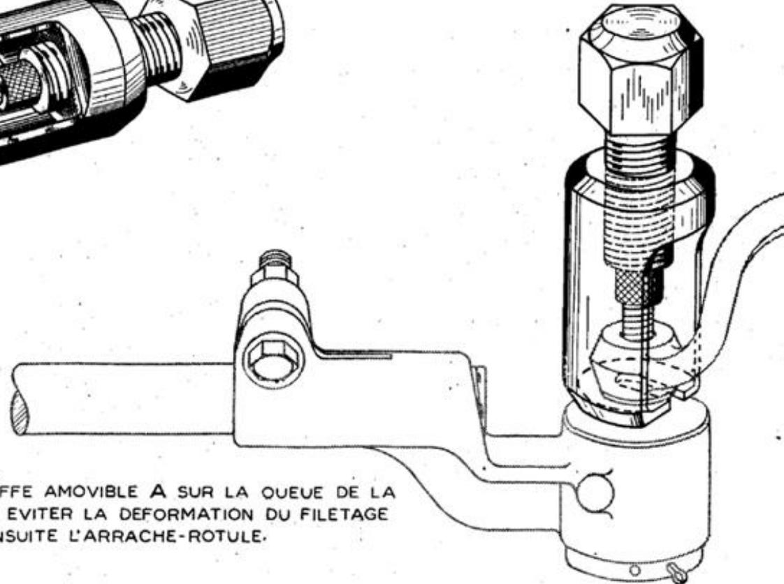
VISSER LA COIFFE AMOVIBLE A SUR LA QUEUE DE LA ROTULE POUR EVITER LA DEFORMATION DU FILETAGE ET PLACER ENSUITE L'ARRACHE-ROTULE.
