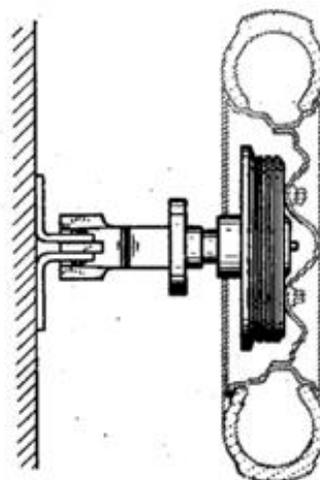
Fig. 3 \_ EMBLACEMENT DES MASSES D'EQUILIBRAGE
