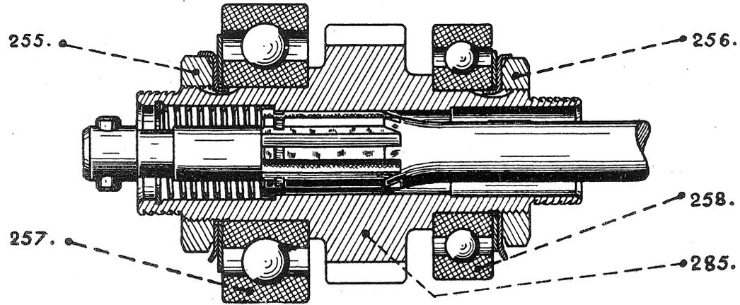
— Fig. 2 — SECTION THROUGH INTERMEDIATE GEAR TRAIN
