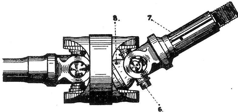
FIG.4. REMOVING DOUBLE YOKE
