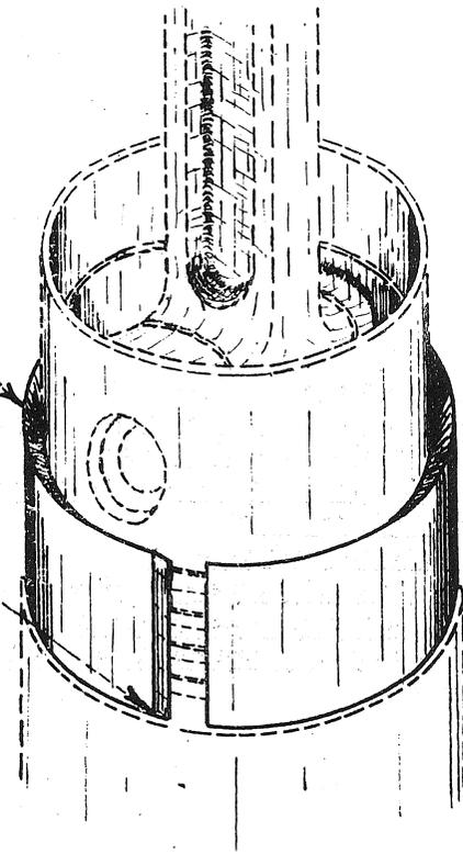
Inner chamfer towards the top to facilitate entry of piston rings in bush.
