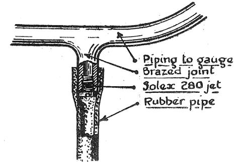
The pump to be tested is fitted on an engine sump and driven by an electric drill at a speed between 1000 and 1500 r.p.m. (Normal speed of machine and usually marked on maker's name plate).
