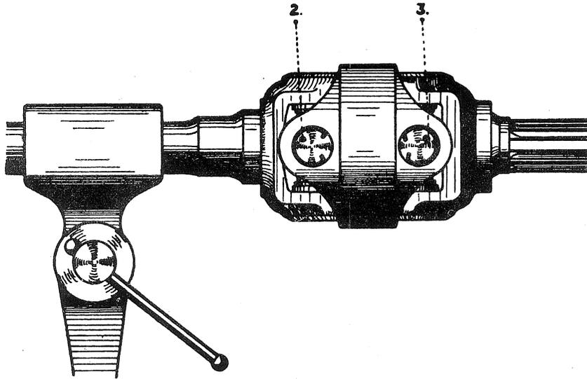
FIG.2. REMOVING NEEDLE BEARING CUPS.
