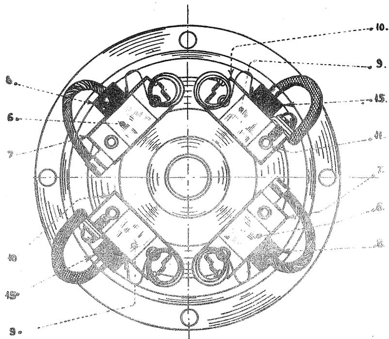
Brushes are held in raised position by springs to allow passage of commutator when fitting armature.
