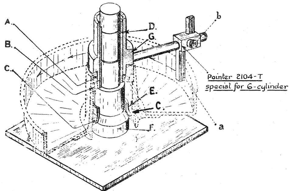
Brake drum equipped with S.P.I. oil seal, complete inner Timken bearing "B", and outer race only of outer Timken bearing "C".
