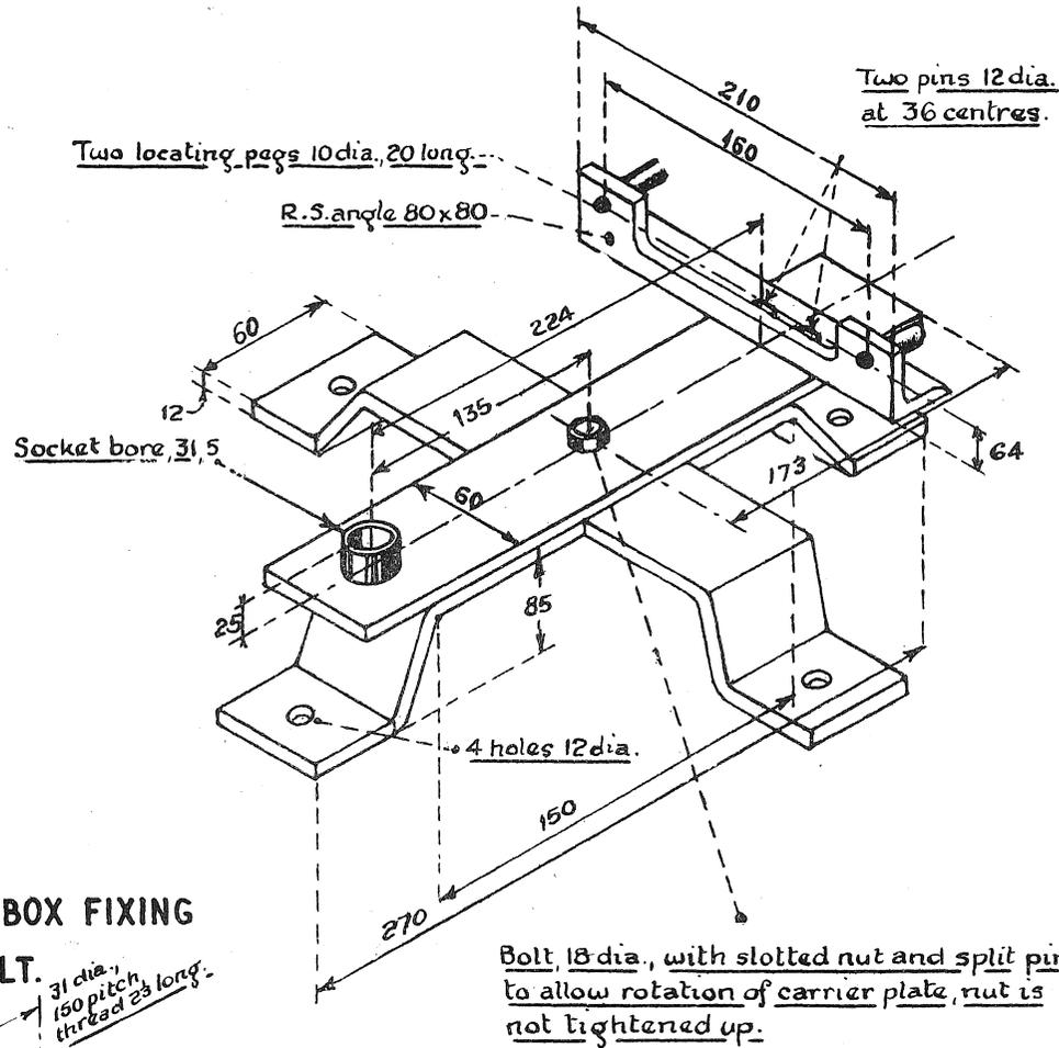
FIG. 3. GEARBOX FIXING
