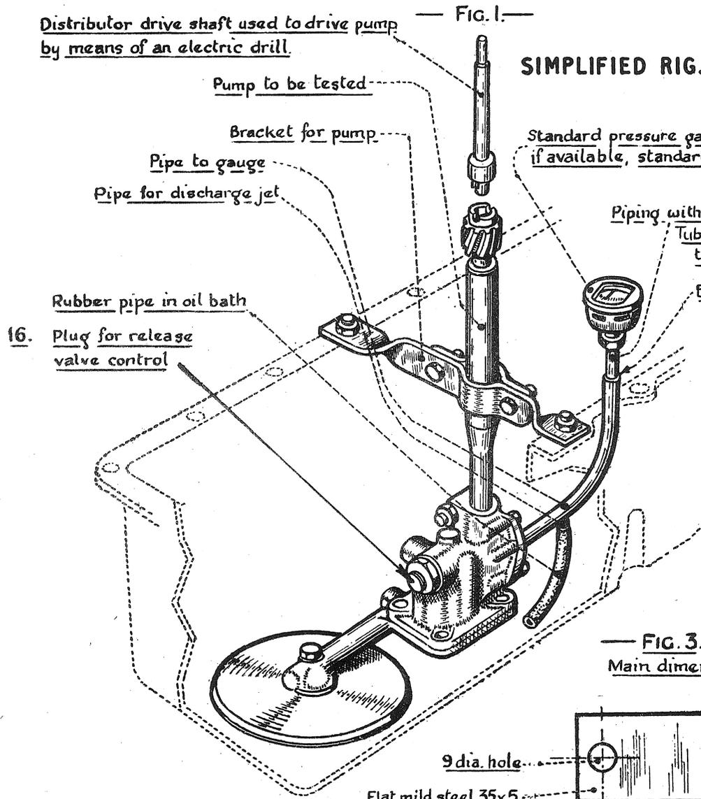
ASSEMBLY OF JET LIMITING DISCHARGE
