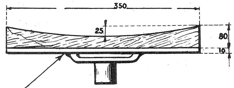
Steel plate welded to standard jack head
