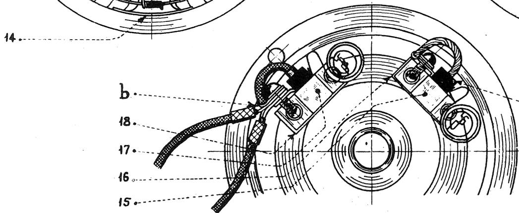
Brushes held in raised position by springs to allow fitting of armature.
