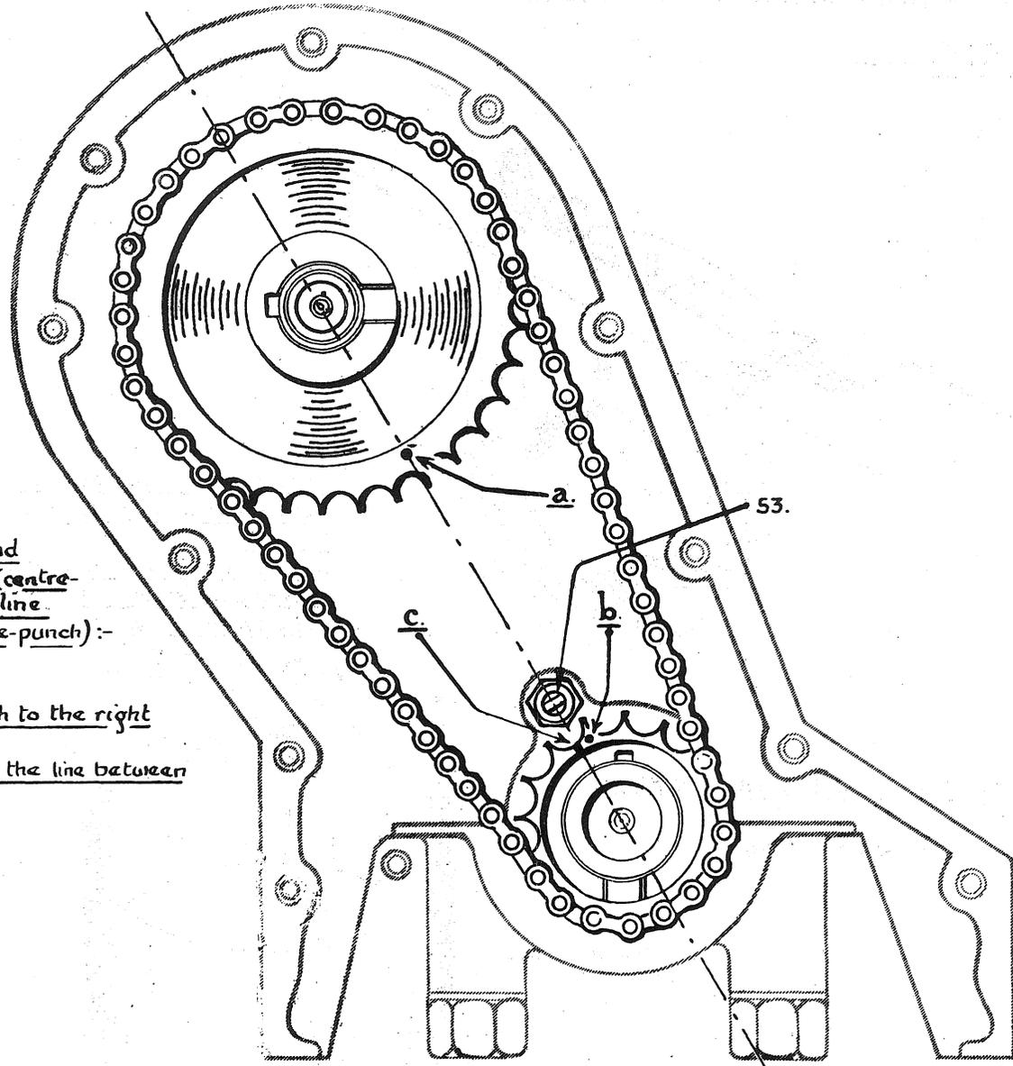
The end cylinders being at approximately top dead centre, the centres of both wheels and mark "a" (centre-punch) on camshaft wheel must be in a straight line.
