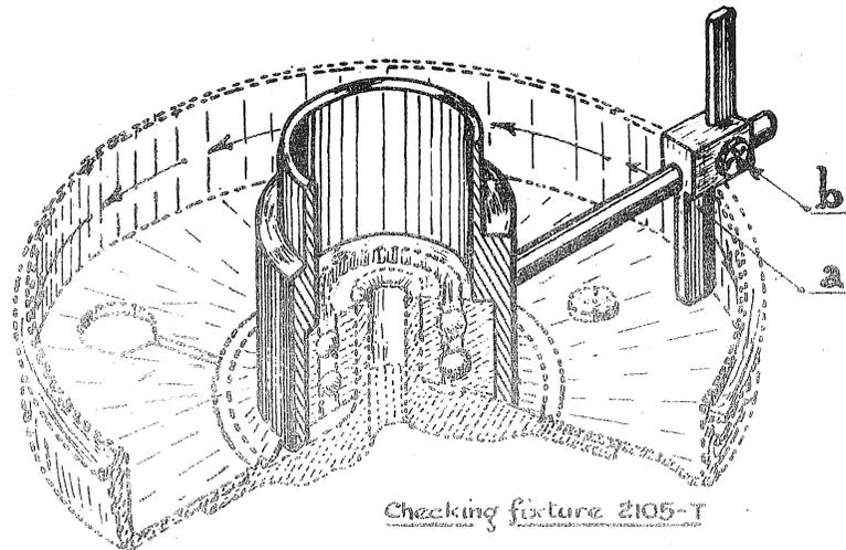
FIG.2. CHECKING CONCENTRICITY OF LININGS.
