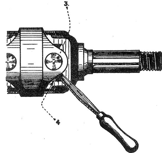
FIG.3. REMOVING STUB AXLE
