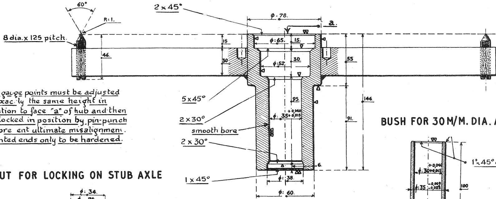
Two gauge points must be adjusted to exactly the same height in relation to face "a" of hub and then be locked in position by pin-punch to prevent ultimate misalignment. Pointed ends only to be hardened.
