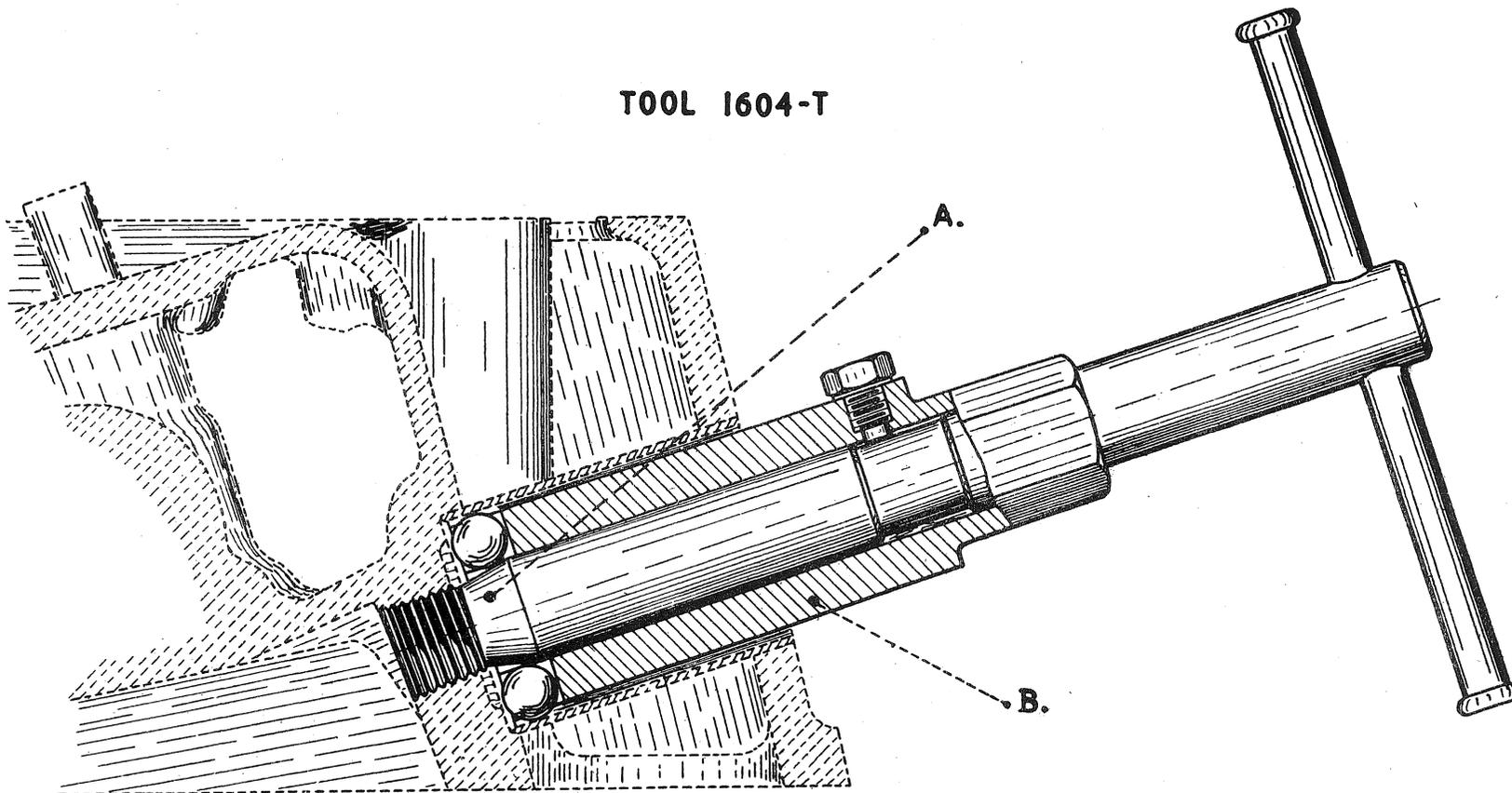
Push body "B" into spark plug housing.
