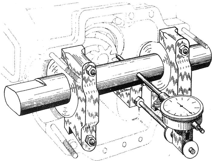
Fig.2 ADJUSTMENT OF MESH
