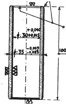
1 x 45° chamfers at both ends
