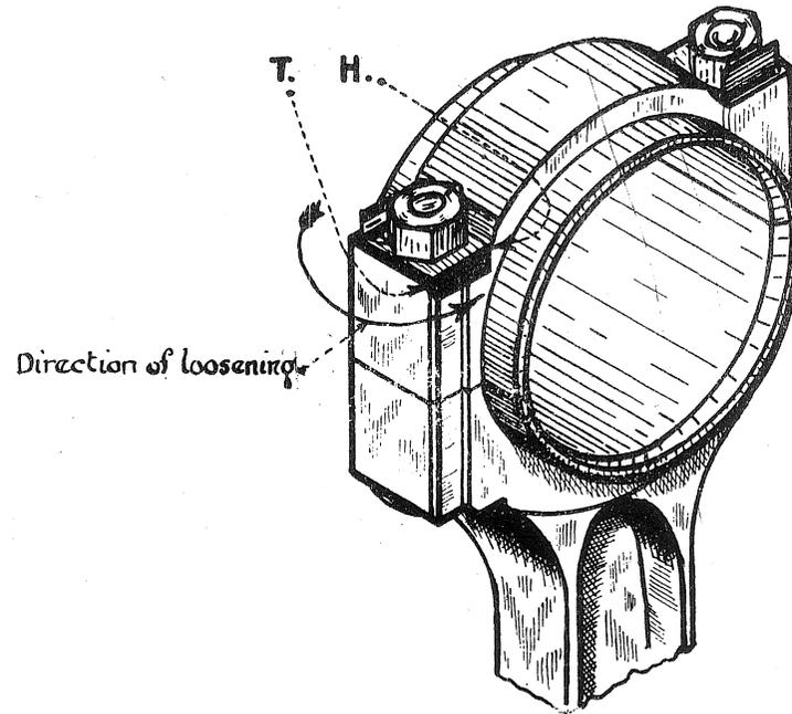
Tab "T" of each lockwasher must butt at "H" in order to prevent nuts turning in the direction of loosening.
