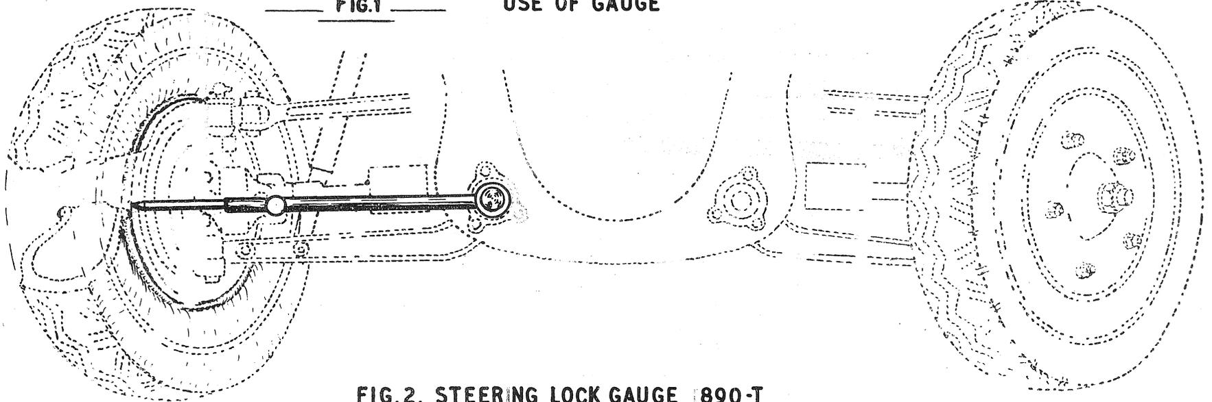
FIG.2. STEERING LOCK GAUGE 1890-T
